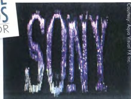
No projection here — the Aqua Visual System uses a computer program to form the water screen's water droplets into company logos and other images.
